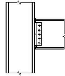
(g) Hybrid (welded flange/bolted web) site connection
