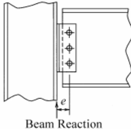
Fig 18.6. Eccentric shear acting on bolt group
