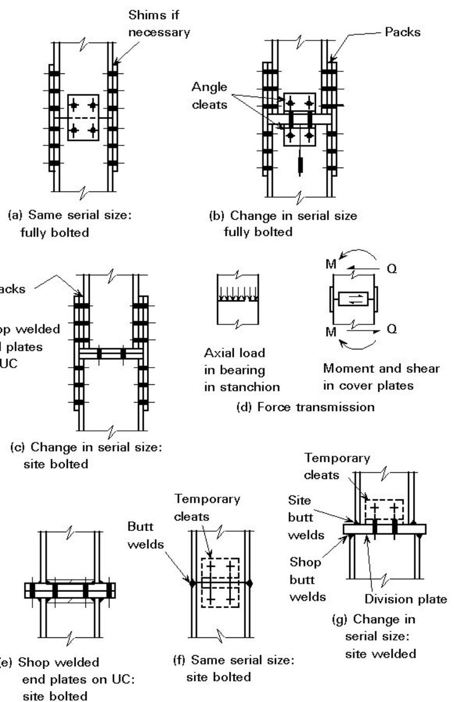
Figure 3 Column splices
