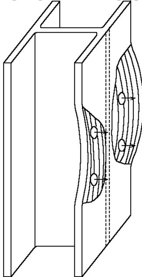
Figure 5 Transfer of tensile force via bending of the column flange in a bolted connection
