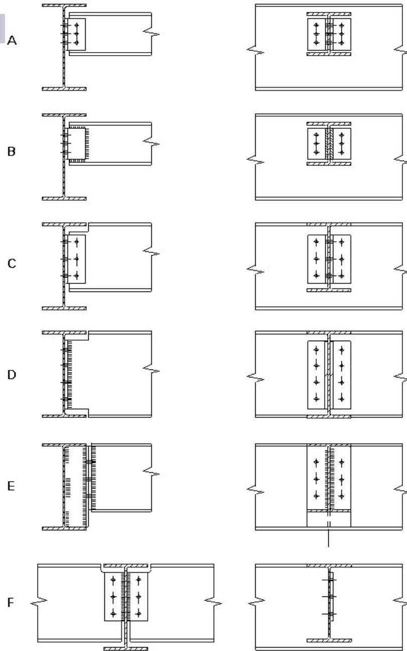
Figure 2 Beam-to-beam connections
