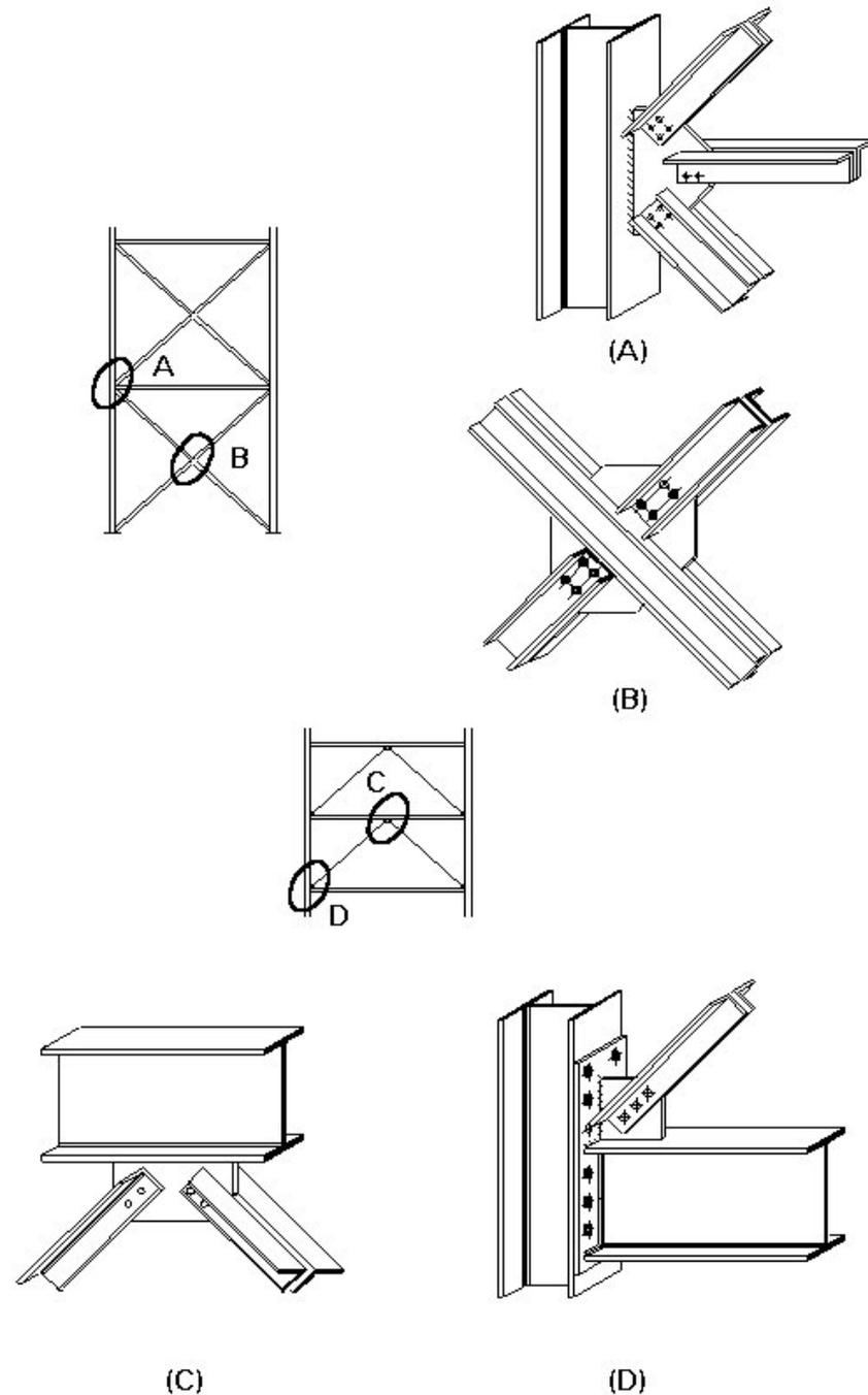
Figure 7 Bracing connections
