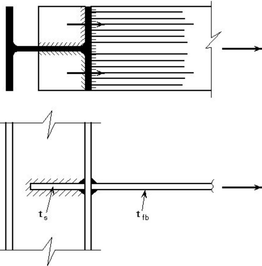
Figure 4 Stiffening plates to strengthen the column flange
