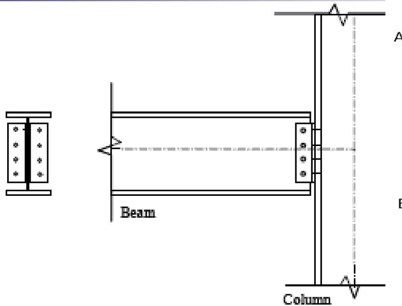
Figure 6. All-bolted double angle shear connection.
