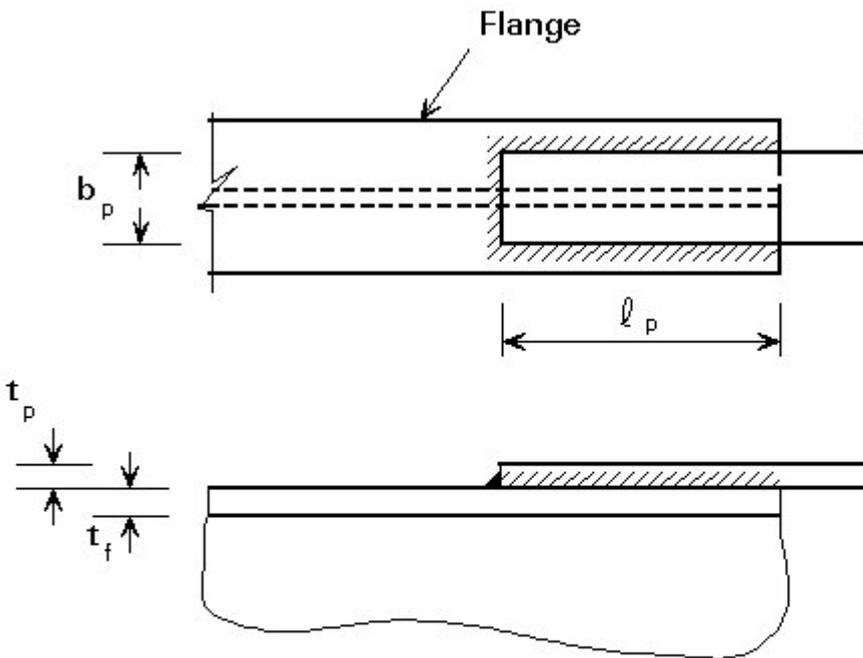
Figure 3 Welded cover plate
