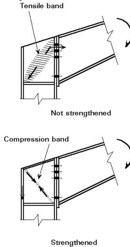
Figure 22 Schematization of the action in the shear zone with tension and compression
