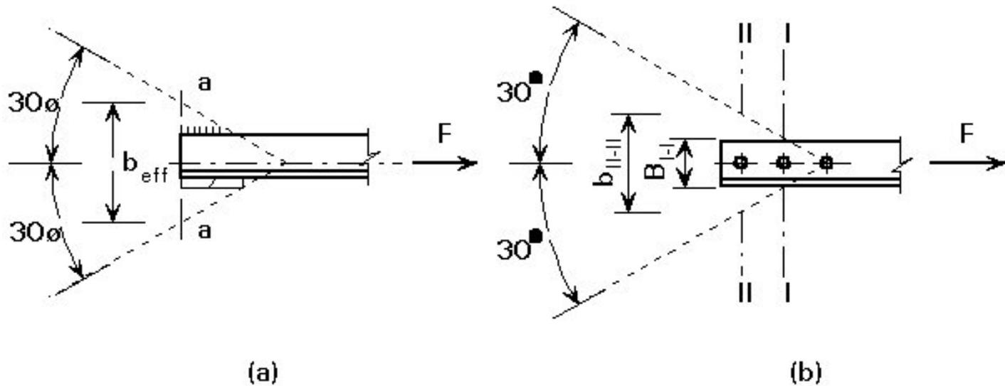
Figure 16 Spread and effective breadth in a welded and a bolted connection
