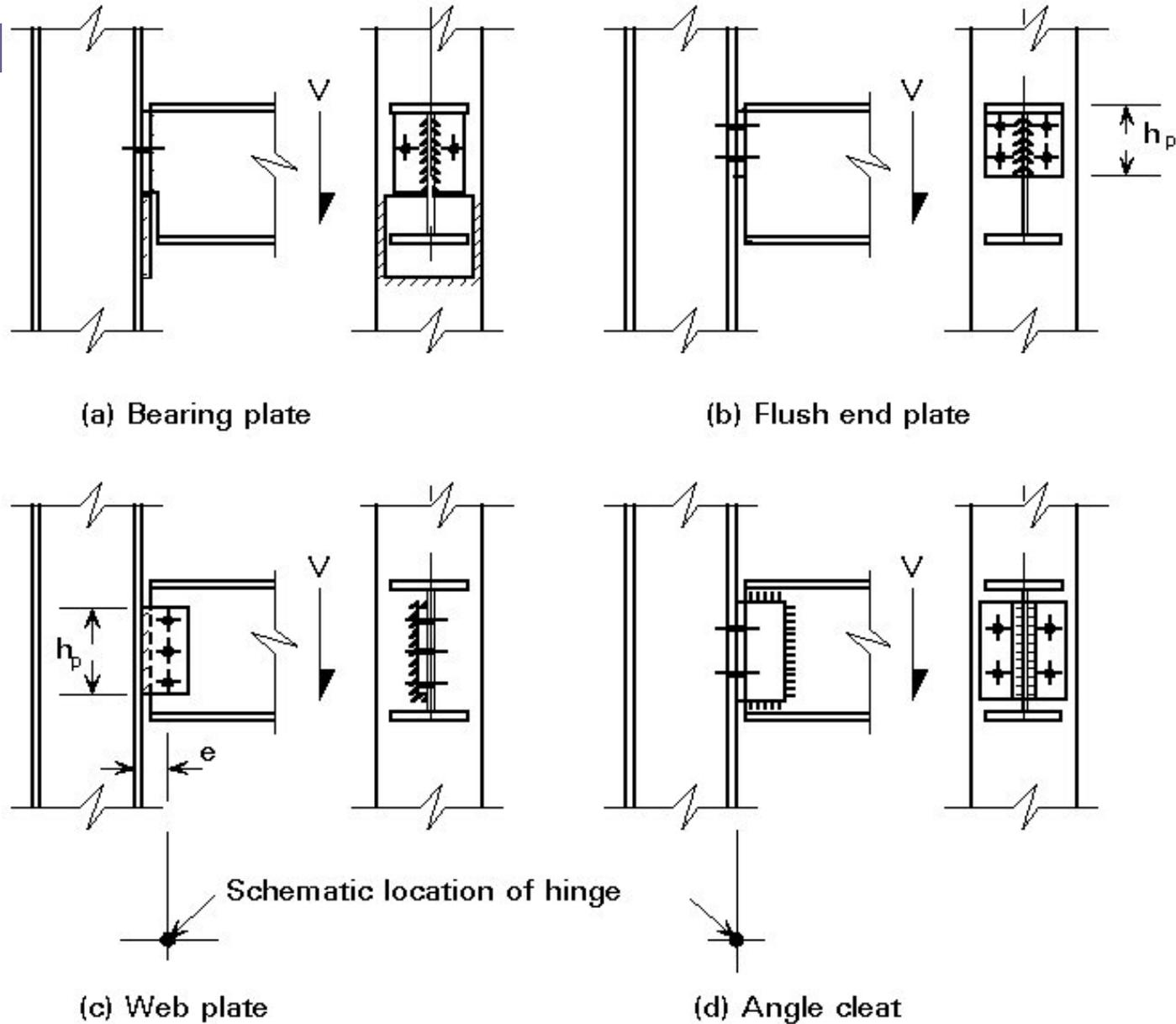
Figure 17 Connections to transfer beam loading into column by means of shear
