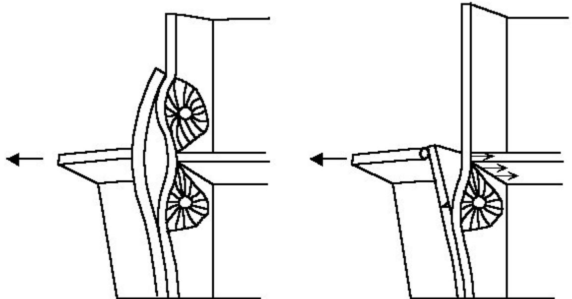
Figure 12 Strengthening the column flange
