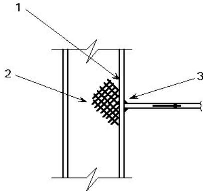
1. Plastic failure of the column flange
