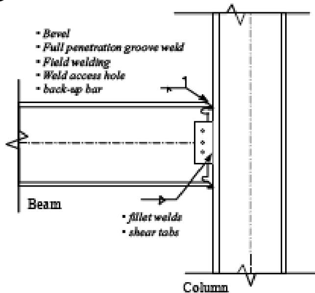
Figure 7. Directly welded flange fully restrained moment connection
