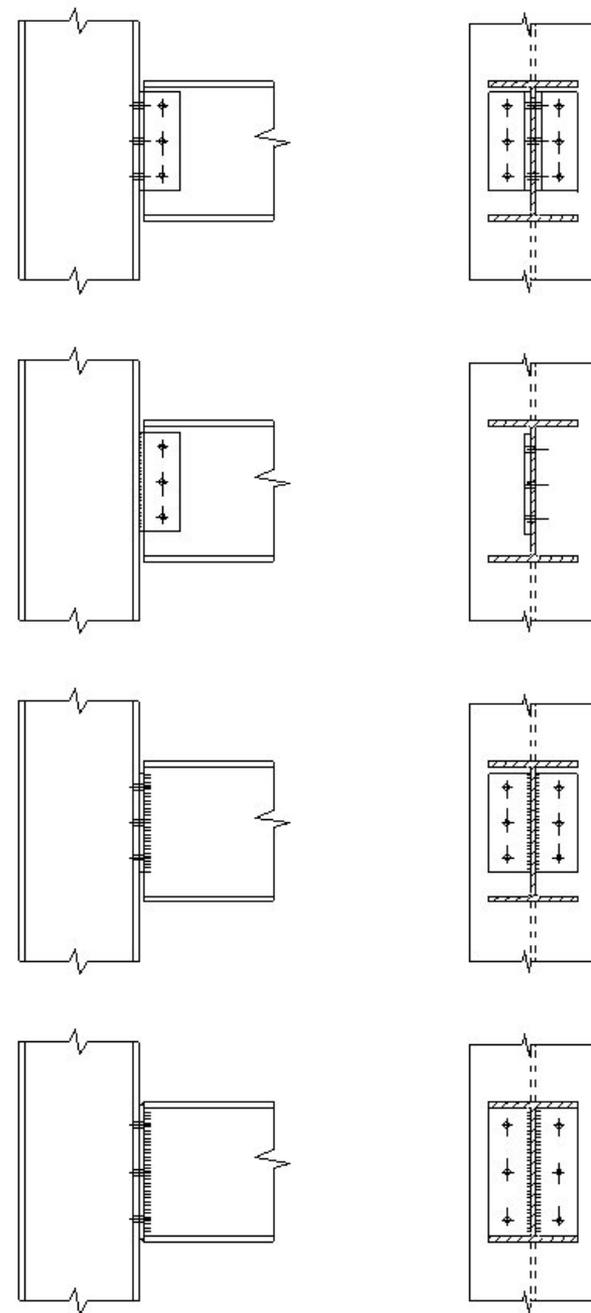
Figure 3. Beam-to-column connections
