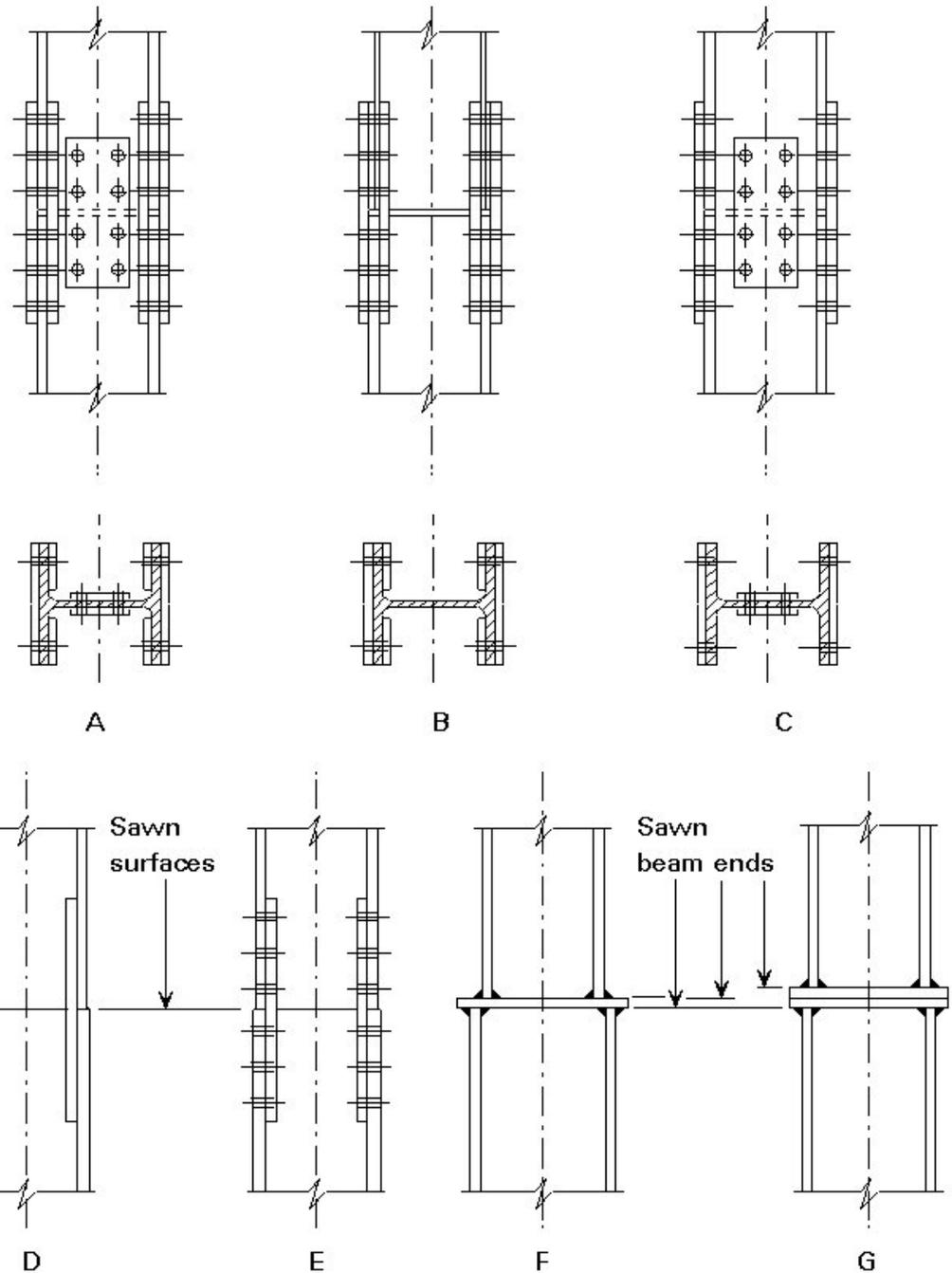
Figure 6 Column splices
