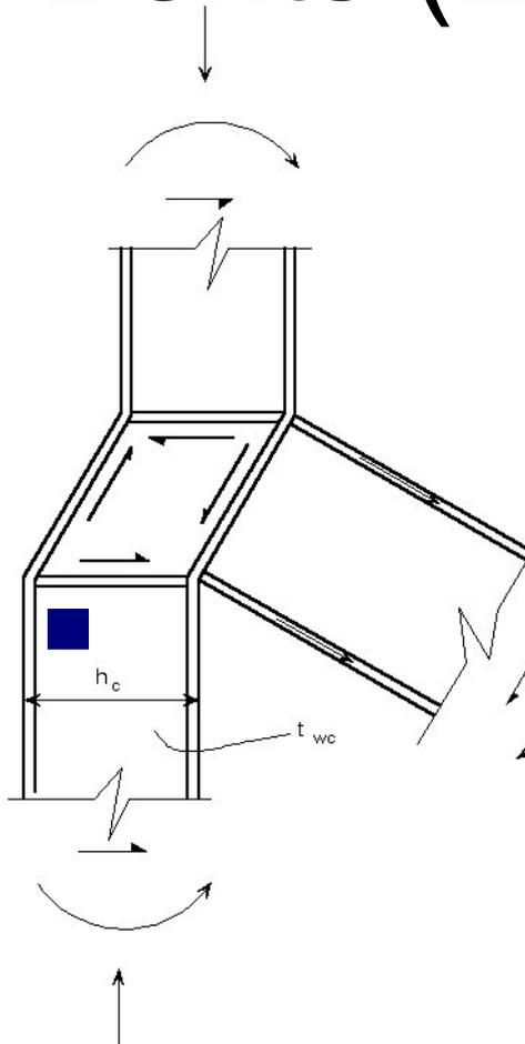
Figure 20 Shear panel of a T-connection
