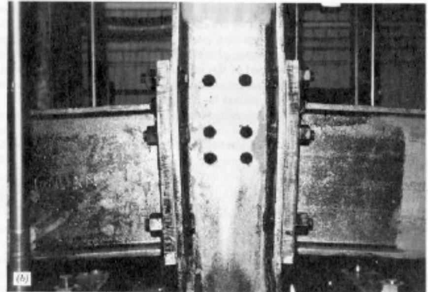
Fig. 18.19. Deformation of column in moment resistant connection. (a) Distortion of unstiffened column. (b) Web crippling in beam-to-column connection. (Courtesy of British Steel Corp.)
