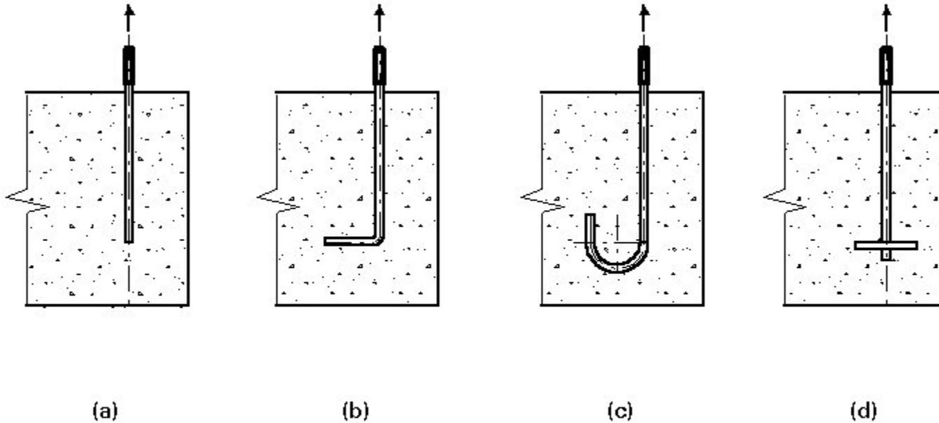
Figure 9 Anchorages of holding down bolts
