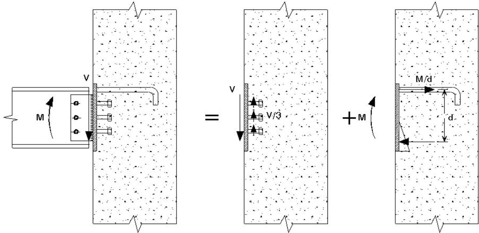
Figure 11 Design model for connection of figure 10(e) subject to shear and moment
