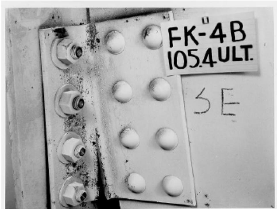
Fig. 18.5. Angle in standard beam connections described in Fig. 18.4. (Courtesy of University of Illinois.)
