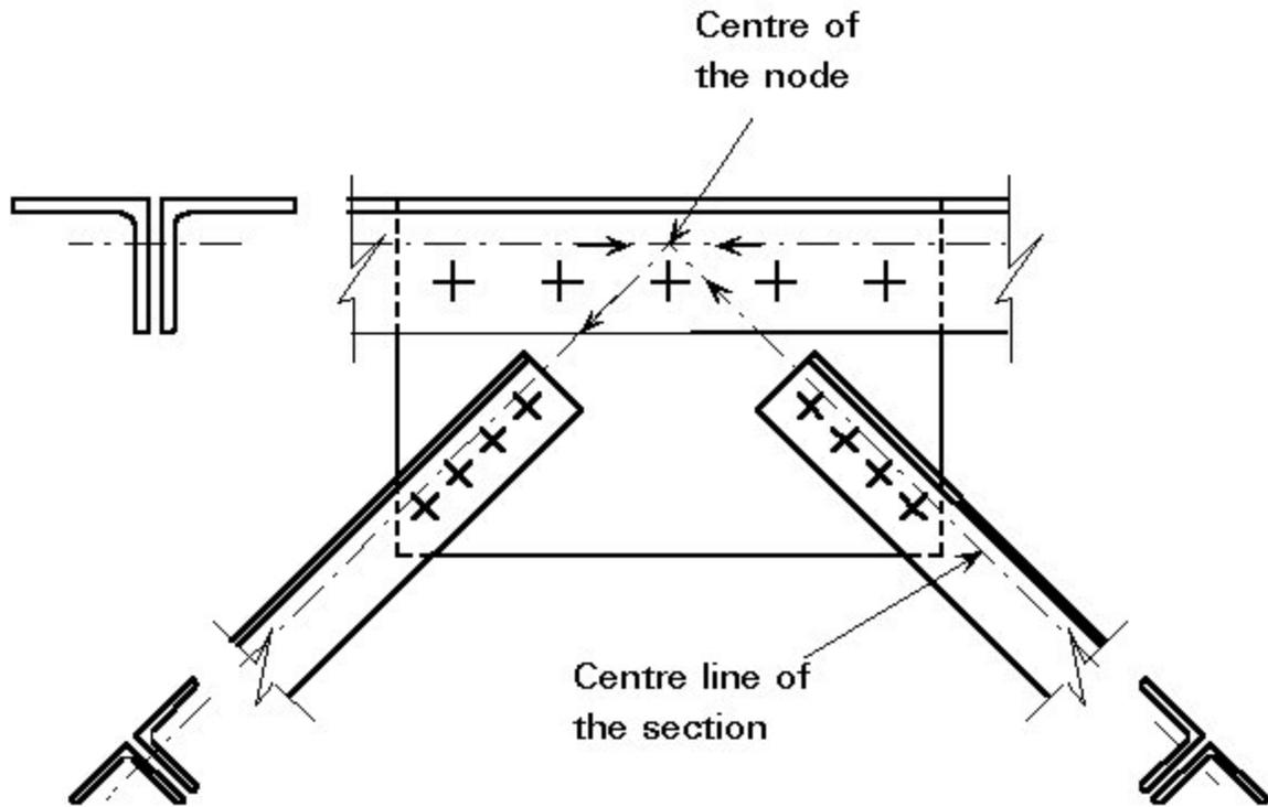
Figure 10 Bolted connection between angles
